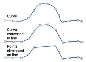
Figure 79: Converting curve to line and eliminating points
