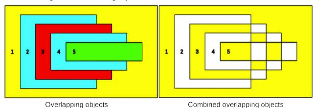
Figure 125: Example of area fill when combining overlapping objects
