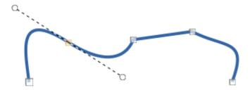
Figure 310: Example of a symmetrical transition point
