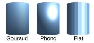
Figure 188: Examples of shading mode
