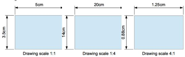
Figure 292: Examples of drawing to scale
